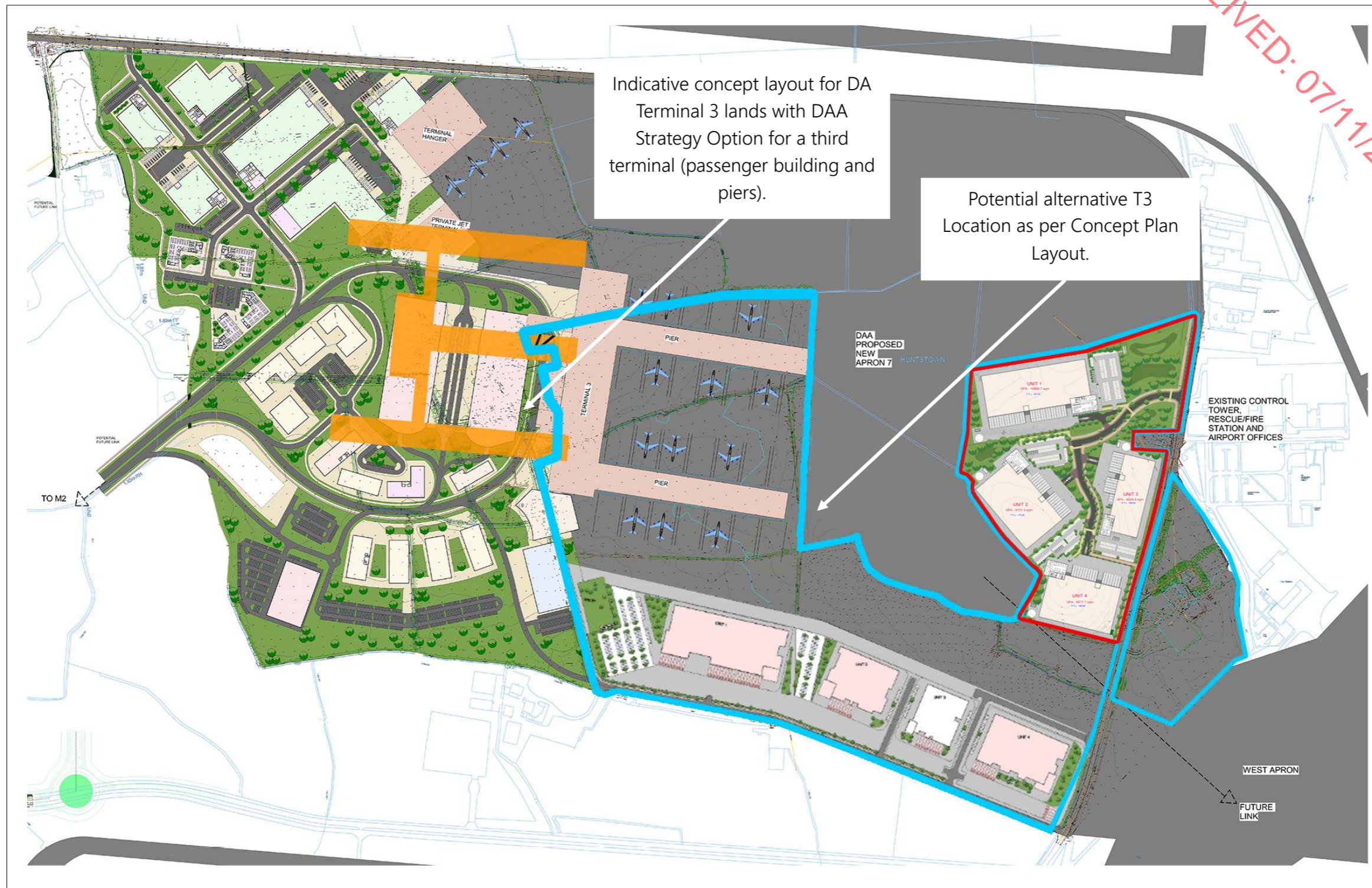
Figure 7: Indicative concept layout for DA Terminal 3 lands with DAA Strategy Option for a third terminal (passenger building and piers).
